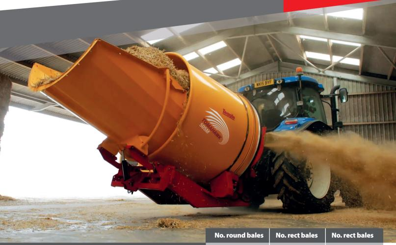
**SUITABLE FOR:** Processing short material for TMR, Cubicles, Poultry Bedding or Biomass
