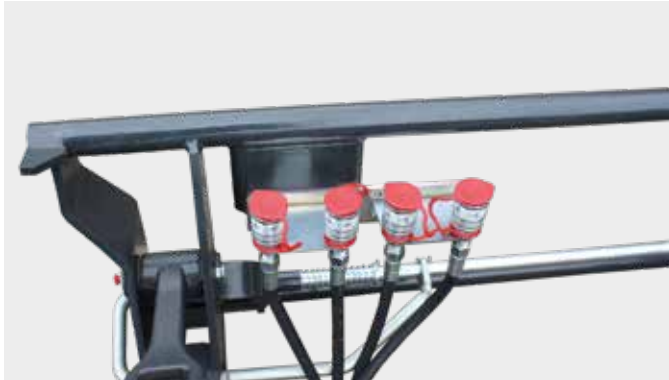
3rd and 4th pilot circuit (here as a plug-in coupling) For the easy operation of hydraulic implements such as silage tongs, bale grabbers or bale stackers.
