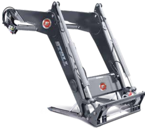
FZ lifting arms with mechanical parallel linkage: Powerful solutions for professionals by professionals
