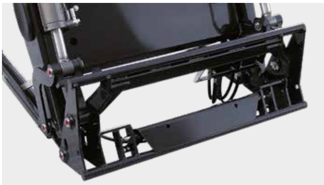
Implement locking mechanism at the touch of a button, making it even more convenient to change the implement without having to get out of the cab – with HYDRO-LOCK.
