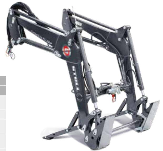
FC-P lifting arms with mechanical parallel linkage
