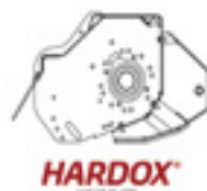
INTERNAL DOUBLE FRAME + STATIC KNIVES IN HARDOX
